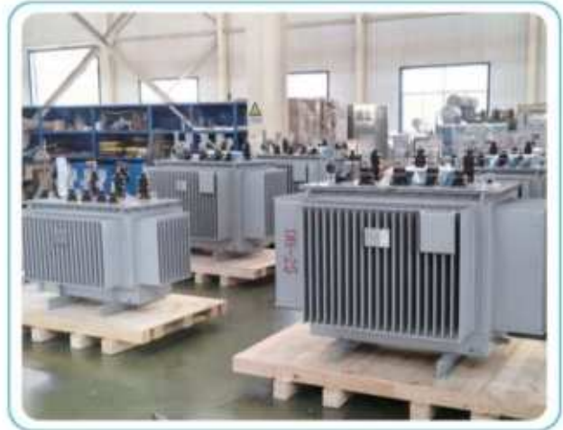
Export to Japan S11- 1000KVA/6.6KV/0.4kV
